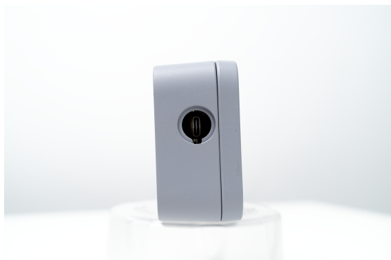
Figure 8: USB Type-C connector access
