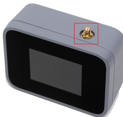
Figure 5: RAK10701-P RP-SMA antenna port
