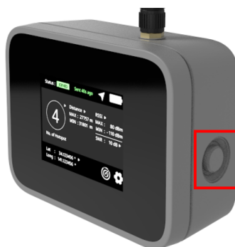
Figure 4: RAK10701-L useable button
